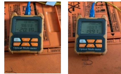
Figure 7 a. FAT 11 uplink attenuation, b. FAT 11 downlink attenuation
