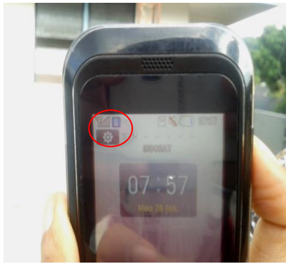
Figure 11. Signal strength displayed as bars on the phone after using the grid antenna.
