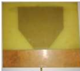
Fig.4 Ground Fabrication Result
