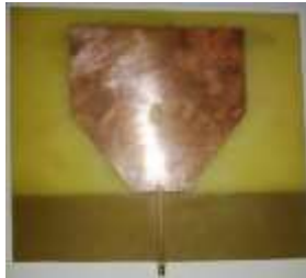
Fig.3 Patch Fabrication Result
