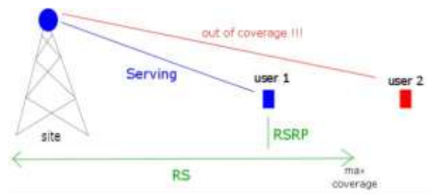
Fig. 2 User Equipment Receives Signal From Site
