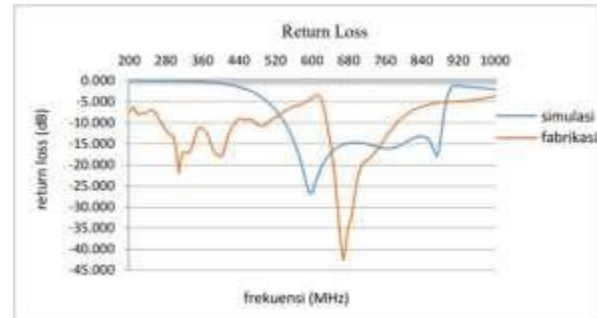
Figure 1 Comparison of Simulated and Measured Working Frequency Graphs.
