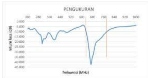
Figure 3 Bandwidth of Measured Antenna
