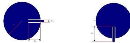
Figure 3. Insert Feed Antena Mikrostrip [10]
